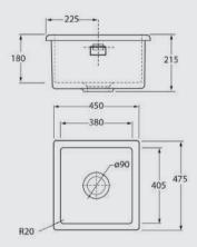
PLEASE NOTE: A DXF is not available, sink should be used as template. When undermounting, a minimum gap of 4mm must be left between the sink and the worktop.
