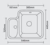
PLEASE NOTE: A DXF is not available, sink should be used as template. When installing, a minimum gap of 4mm must be left between the sink and the worktop.
